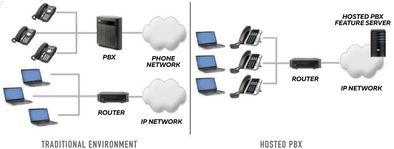
*In a traditional environment, multiple connections are required to deliver voice and data, and multiple pieces of equipment are needed. With Hosted PBX, a single IP connection delivers everything you need for voice and data, including the phone system functionality.*
